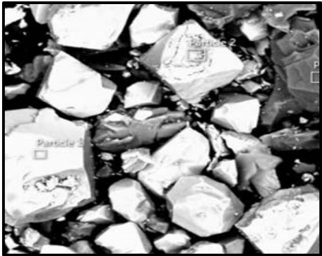
Elutriation removes free silica upgrade > 69%Fe
