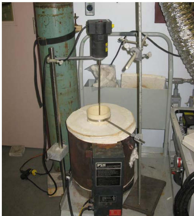
FIGURE: Test work setup for agitated roast vessel
