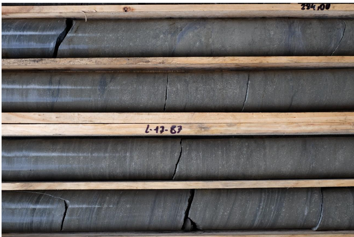
Figure 1: Massive sulphide (upper three rows) and banded semi-massive sulphide (lower row) in DDH L17-87.
