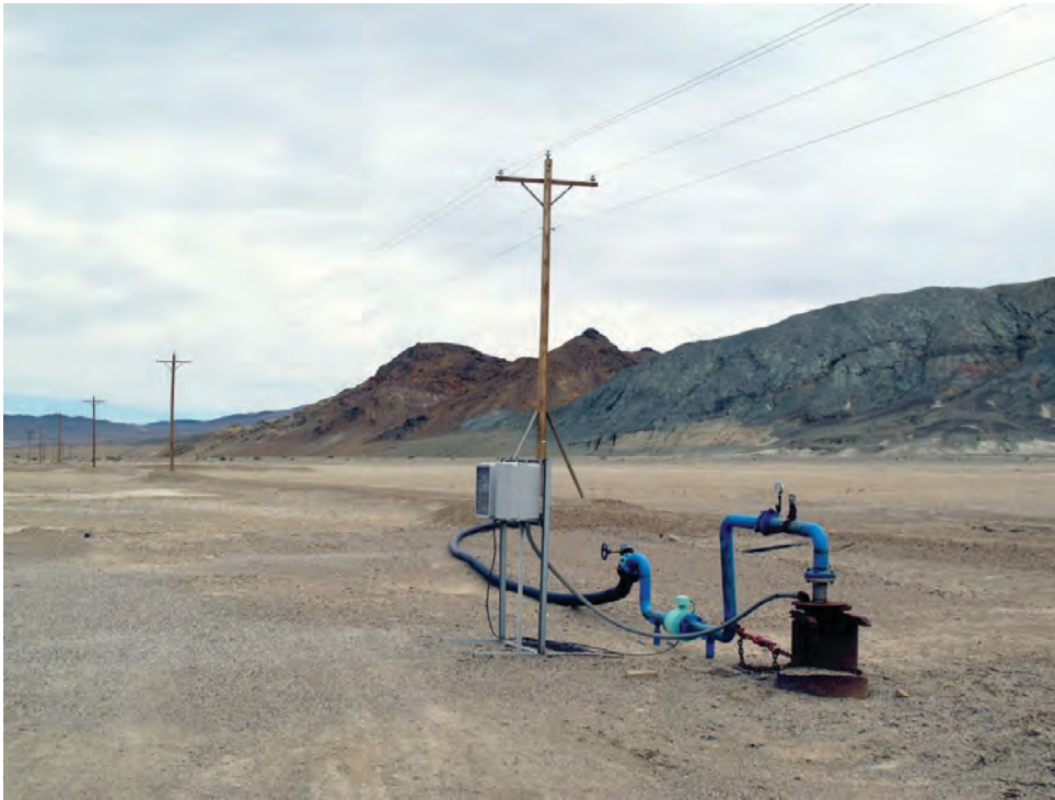
Figure 10: A production well at the Silver Peak operation. The rock face in the background is the fault plane of the Angel Island Fault, against which brines have ponded at depth and which the bore hole in the foreground is targeted.
