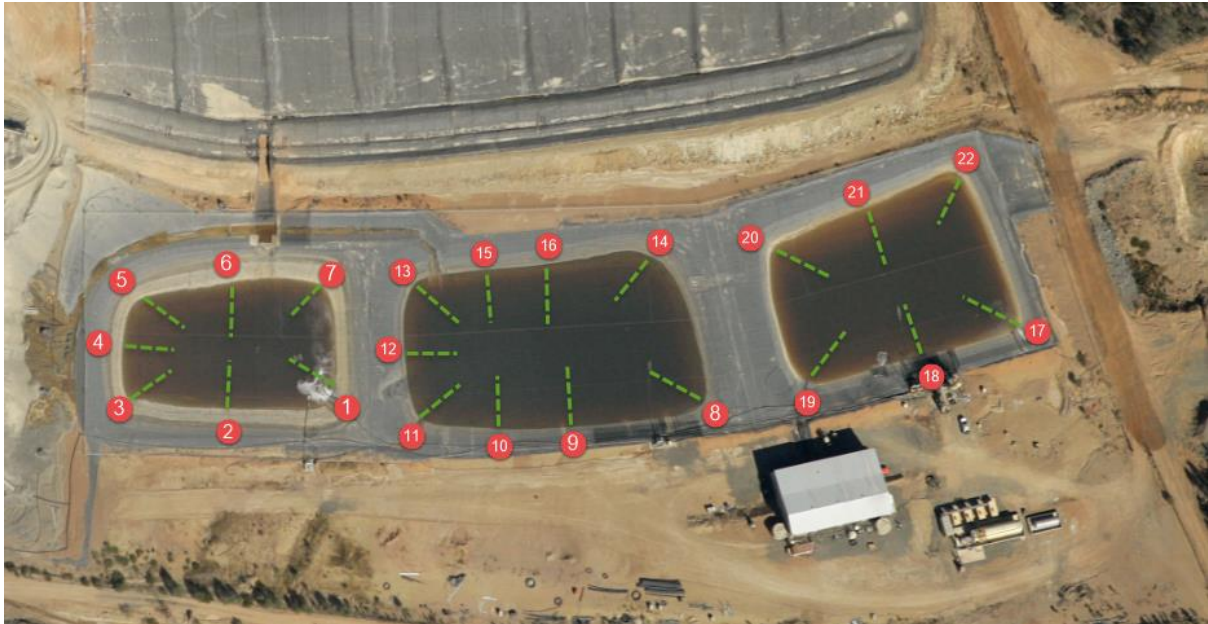
Figure 1: Photo-plan depicting the position of the Pregnant (far left), Intermediate (middle) and Barren (far right) Ponds respectively. Green broken lines depict the sampling traces (approximately 13 long, along the base of the ponds); the coloured spots indicate the sample reference. Scale: 1: 25.
