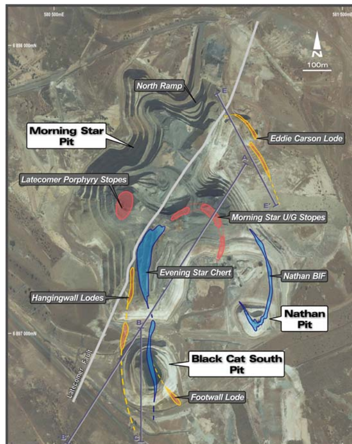
Figure 6: Plan view over the Morning Star and Black Cat South pits highlighting long section traces, through Black Cat South (B – C) and the Morning Star Deeps (A – B)
