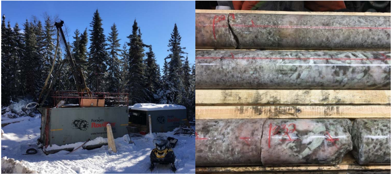
Figure 5: Diamond drill rig on site (left) and diamond core AL-17-005 showing coarse grain spodumene crystals at 229 to 232 metres depth (right)
