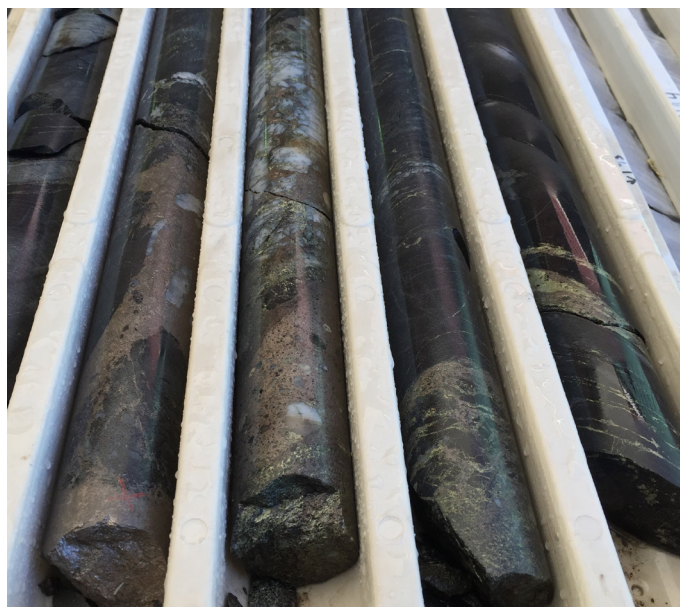
Figure 2: Drill core from hole EL16D05; 195.12-199.63m containing breccia and vein hosted chalcopyrite (yellow) and pyrrhotite (bronze) mineralisation.
