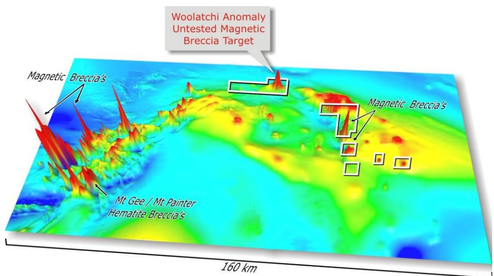
[Figure 1] Frome Joint Ventures, Callabonna Project: 3D oblique view of total magnetic intensity highlighting the large amplitude Woolatchi breccia target which remains to be drill tested.
