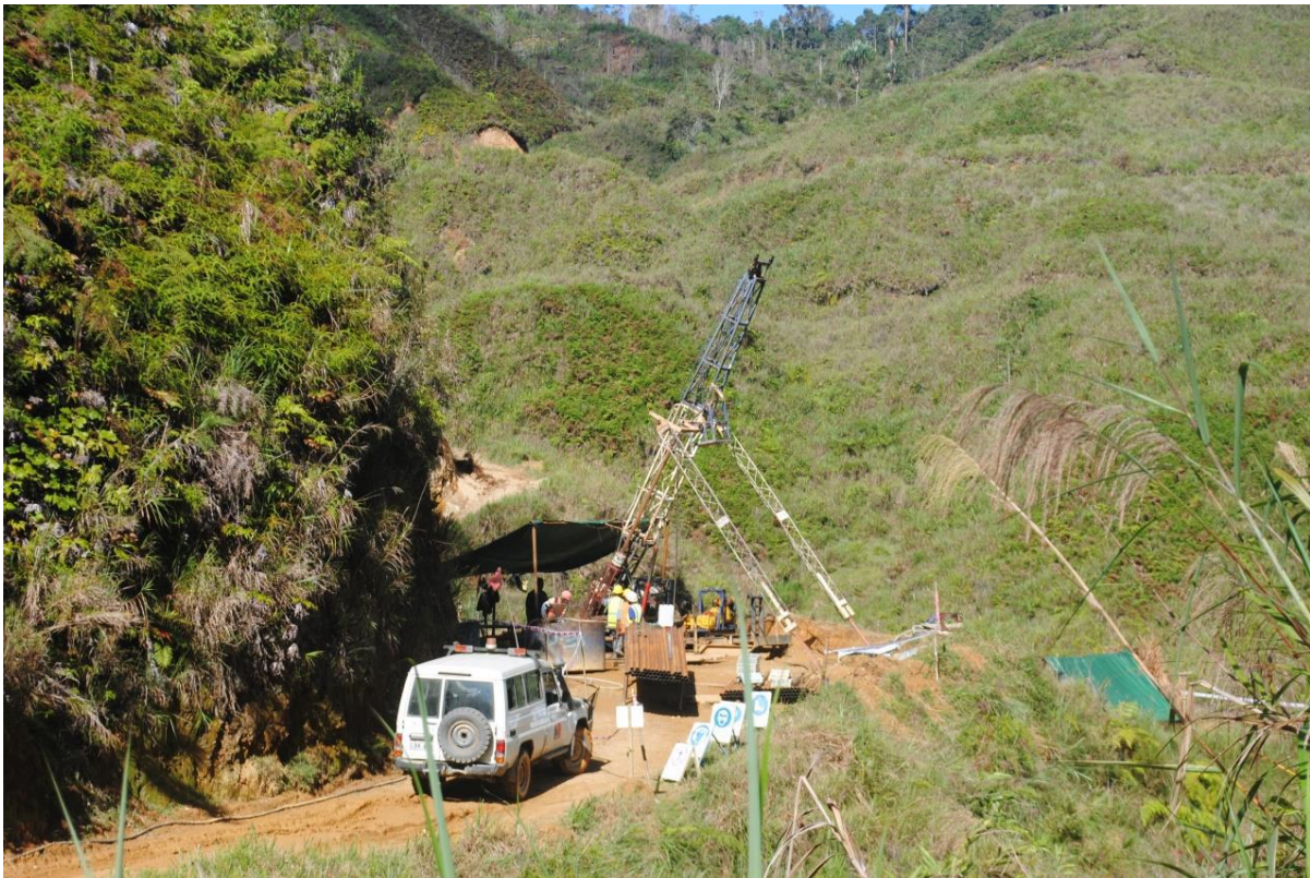
Figure1: Niuminco drill rig and team drilling hole EDD 024 at the Karuka/Enterprise stockwork and diatreme.
