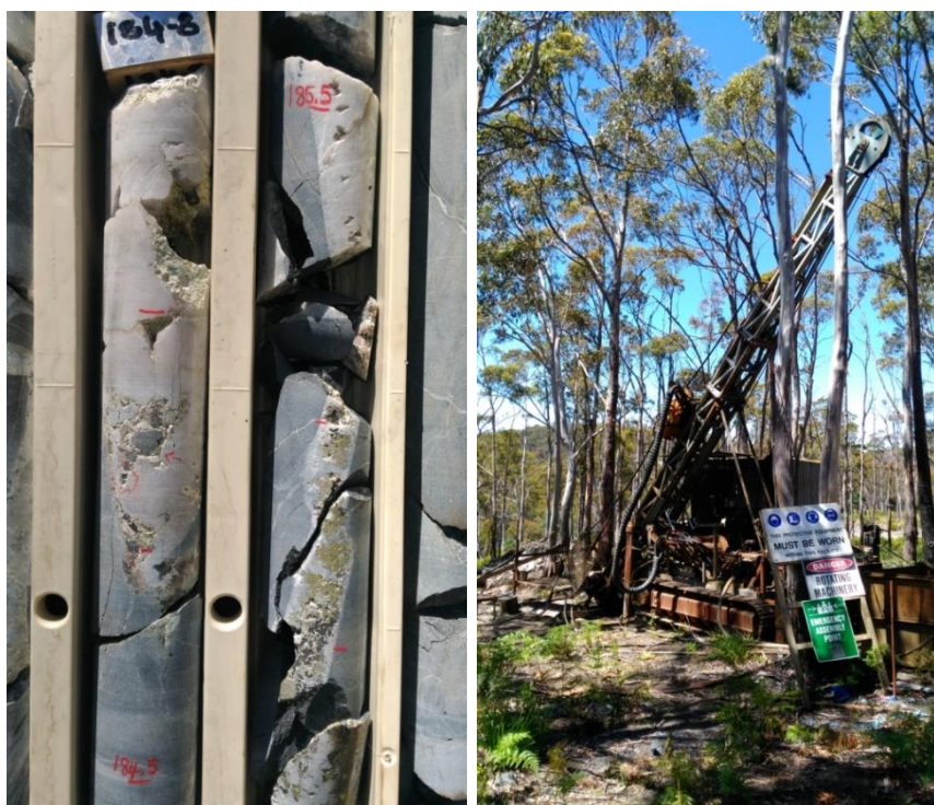
Photo: (Left) coarse grained cassiterite at 184.65m and quartz chalcopyrite-wolfram at 185.35m. (Right) LDD002, view to SSE
