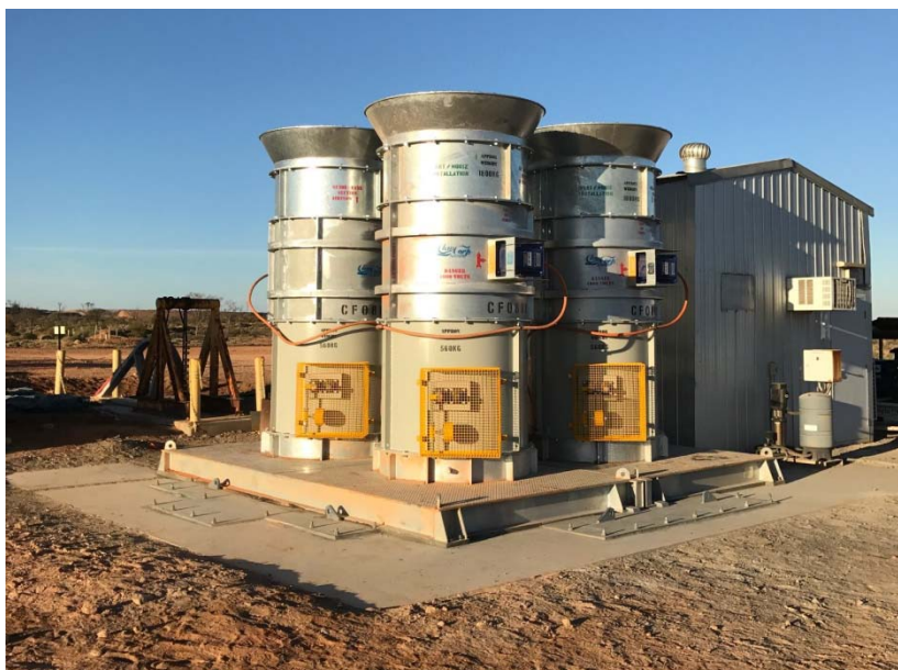
Figure 1: primary fan bank at the ventilation shaft collar fully installed and running
