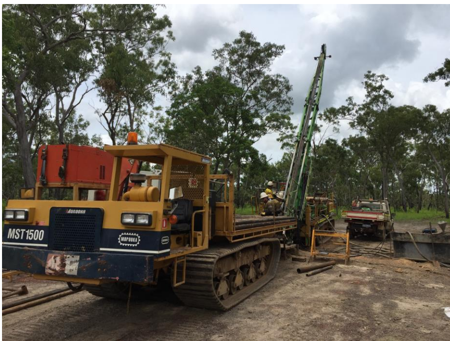
Figure 3. Track-mounted diamond rig at Grants Prospect January 2017, Finniss Lithium Project, NT.
