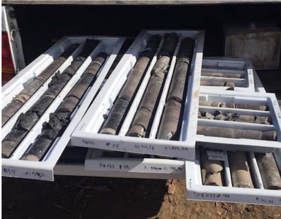
Figure 3: Drill core samples from the current drilling program being undertaken at the Pico Quemado coal project
