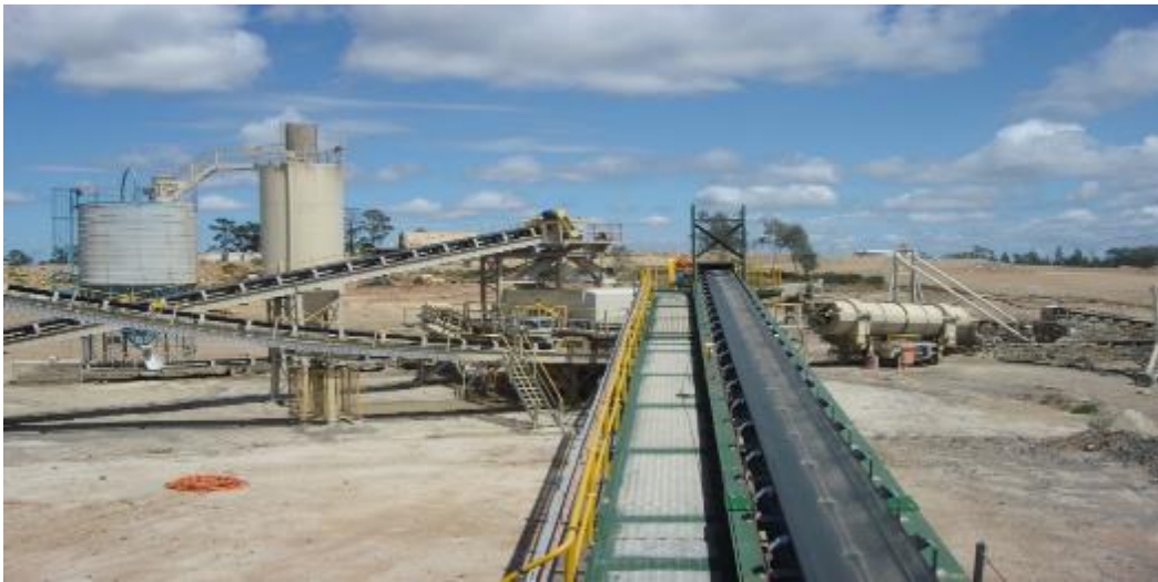
Figure 12: Crushing and screening plant including agglomerator, cement/lime storage silos
