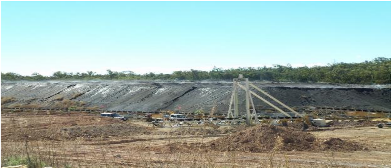
Figure 18: Heap Leach Pad under Irrigation
