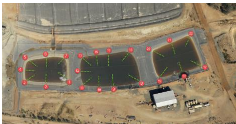
Figure 1: Photo-plan depicting the position of the Pregnant (far left), Intermediate (middle) and Barren (far right) Ponds respectively. Green broken lines depict the sampling traces (approximately 13m long, along the base of the ponds); the coloured spots indicate the sample reference. Scale: 1: 25.
