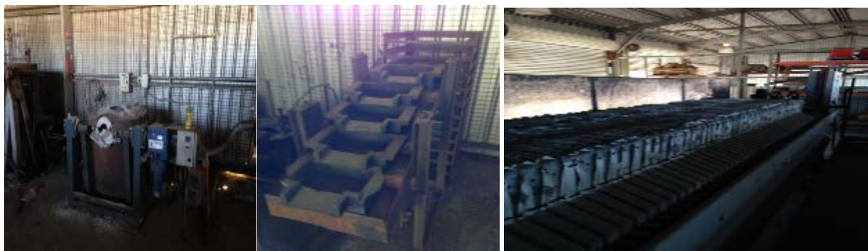
Figure 20: Silver furnace (x2), dore bar ingots and Merrill Crowe plate filter
