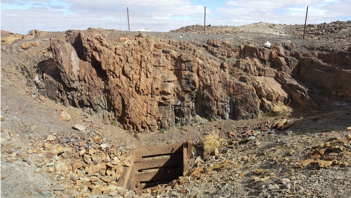
Plate 1. Old mine workings at Copper Blow. Stenhouse Shaft. Mineralised structure is 7 metres wide here.
