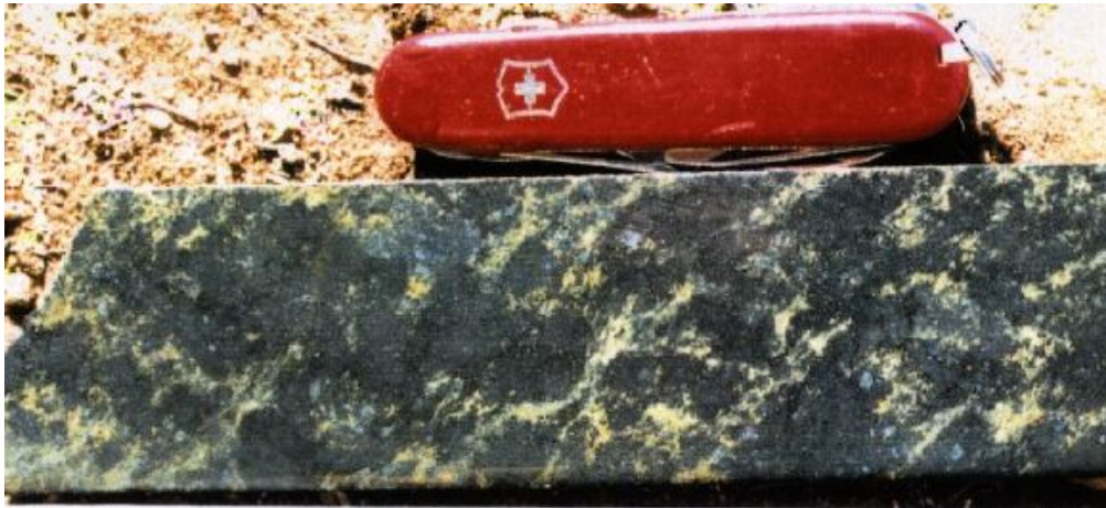
Plate 2. Chalcopyrite and pyrite (yellow) forming infill around replaced clasts of magnetite (black). DDHCB006 at 116.6 metres; part of intersection 116.0m to 120.4m; 4.4m at 2.8% copper and 0.5 g/t gold in the Warren Lode. Photo extracted from Open File Report GS1996/055.
