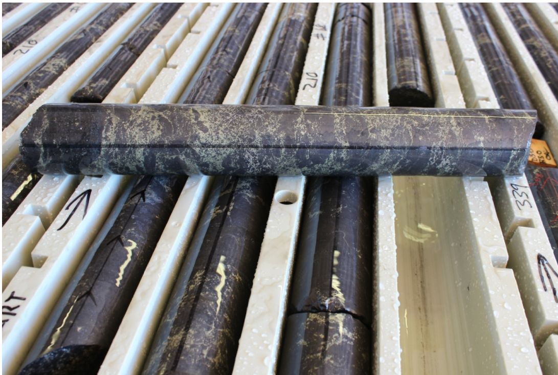
Photograph 6 - Mineralised diamond drill core from KJCD210 (circa 338m) showing interpreted Conductor 3 stringer and disseminated mineralisation in massive magnetite
