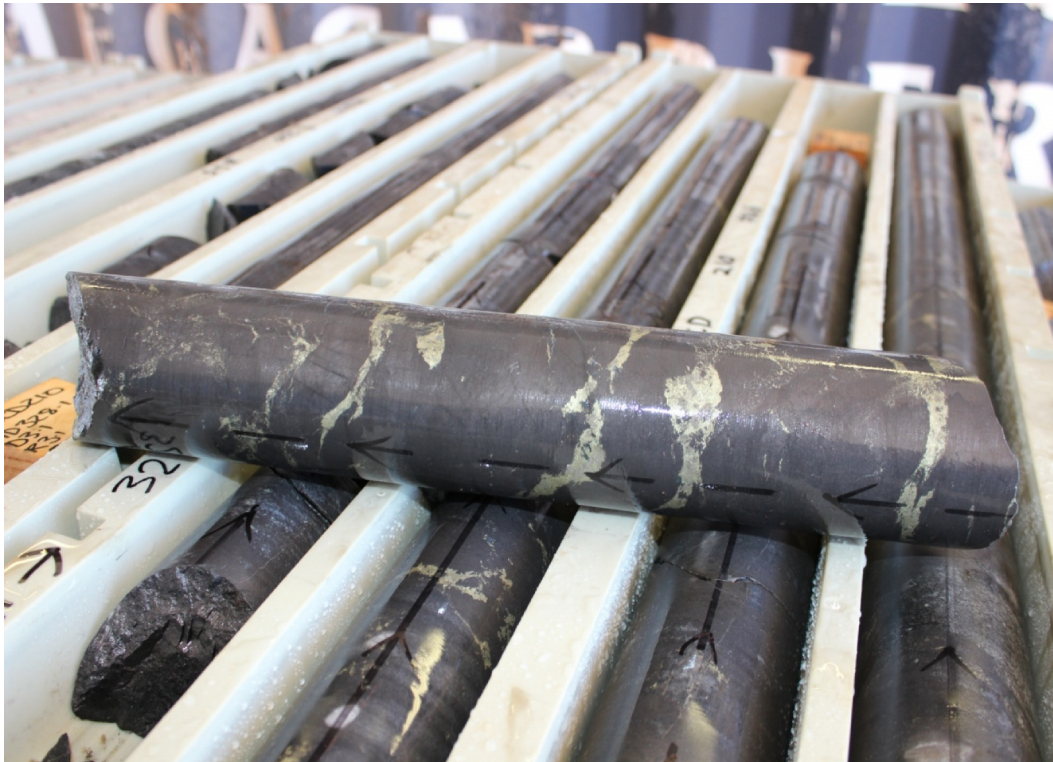
Photograph 5 - Mineralised diamond drill core from KJCD210 (circa 327m) showing interpreted Conductor 1 massive and disseminated sulphide mineralisation in massive magnetite
