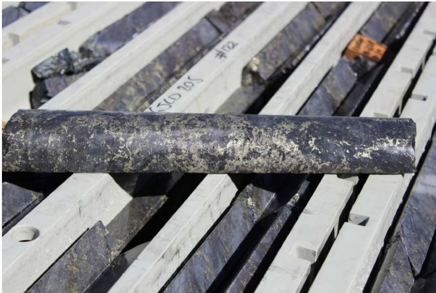
Photograph 2. Mineralised core from KJCD205 (circa 621m) showing chalcopyrite-pyrite sulphide that is hosted within a strongly silica-garnet-magnetite altered host rock (Conductor 5)
