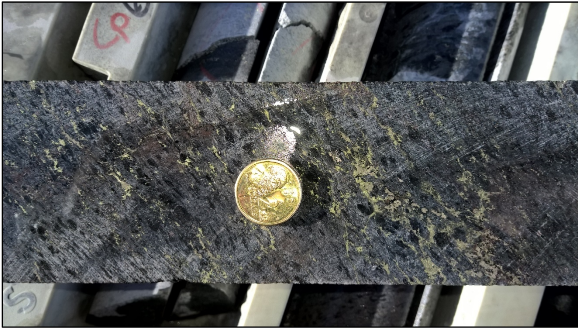
Photograph 4 - Mineralised diamond drill core from KJCD208 (circa 670m) showing interpreted Conductor 7 stringer and disseminated mineralisation
