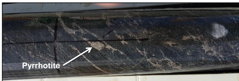
[Figure 1] Woolatchi WO-17-01, Callabonna Project: Core photographs showing iron sulphide (pyrrhotite) and minor copper sulphides as veins and disseminations along shears or vein stock works associated with strong biotite and magnetite alteration
