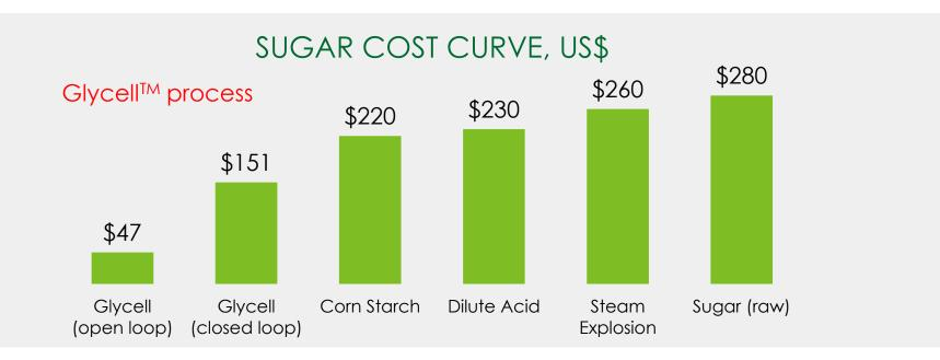
Glycell<sup>TM</sup> closed loop is when the recovered glycerol is recycled. Glycell<sup>TM</sup> open loop is when the recovered Glycerol is sold at a profit. Steam explosion and dilute acid costs from Lux Research. Corn starch from Jacobs Engineering.
