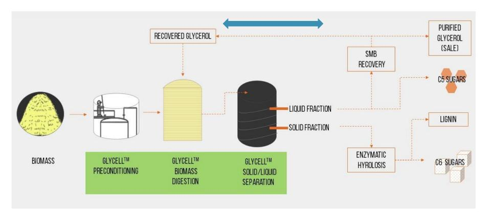
Leaf's Glycell™ process uses waste glycerol from biodiesel manufacturing as the main reagent to break down plant biomass.
