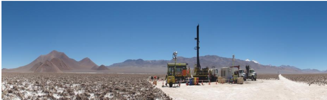
Figure 8: Sonic drilling rig operating at the Maricunga salar
