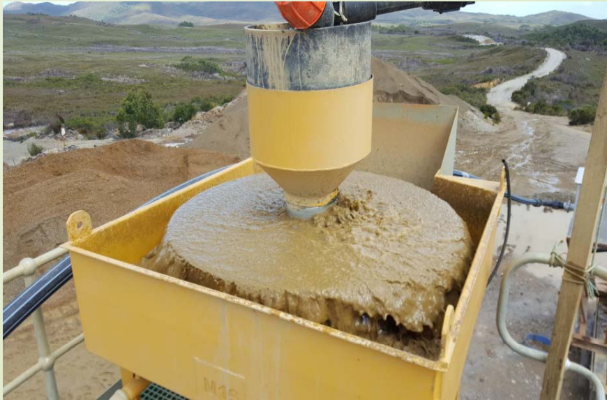
Primary gravity jig (above) and improved recovery since commissioning (below)
