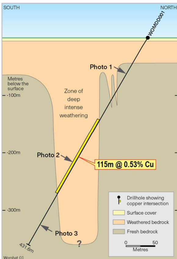
**Figure 3:** Wombat section showing weathering trough.
