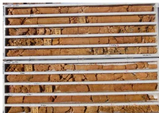
**Photo 2:** WOMDD001 core 253-267m downhole. Porous, permeable, mineralised material.
