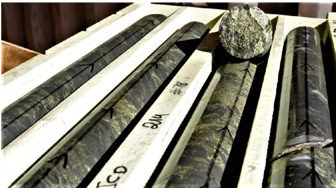
Photograph 2. Hole KJCD214 Zone of semi-massive and breccia of magnetite + chalcopyrite circa 422.6m.
