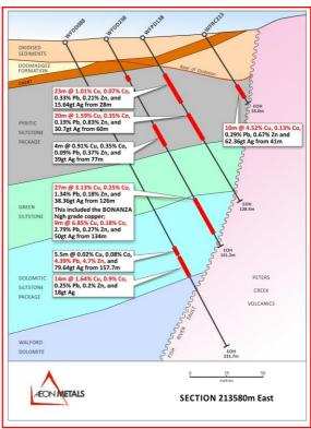
Figure 4: Geological Section for hole WFDD 237 on 213605E and WFDD238 on 213580E
