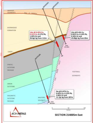
Figure 5: Geological Section for hole WFDD 239 on 213530E and WFDD241 on 214005E
