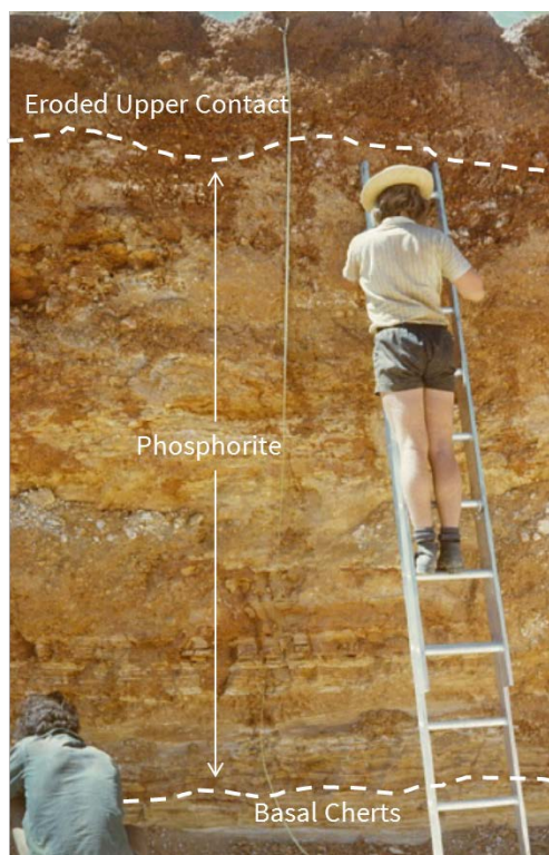
FIGURE: Mapping phosphorite section at Ardmore in excavation (trench) AE4.
