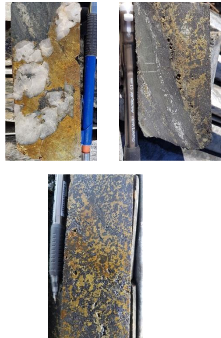
Figure 7. Examples of high grade copper mineralisation. Combinations of chalcopryite, pyrite, magnetite, biotite and quartz.
