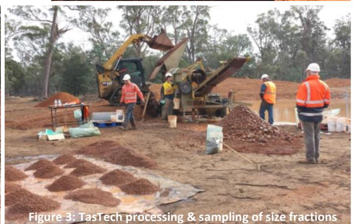
Figure 3: TasTech processing & sampling of size fractions
