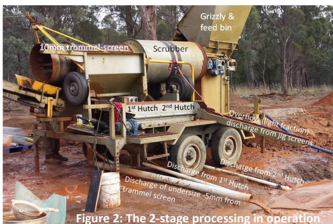
Figure 2: The 2-stage processing in operation
