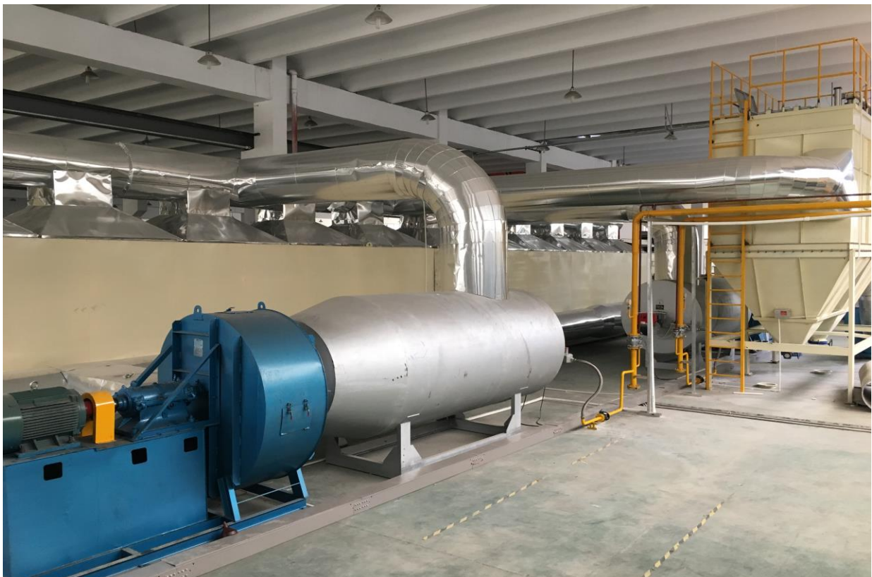
Changxing Factory - gas dryer and bagging facilities
