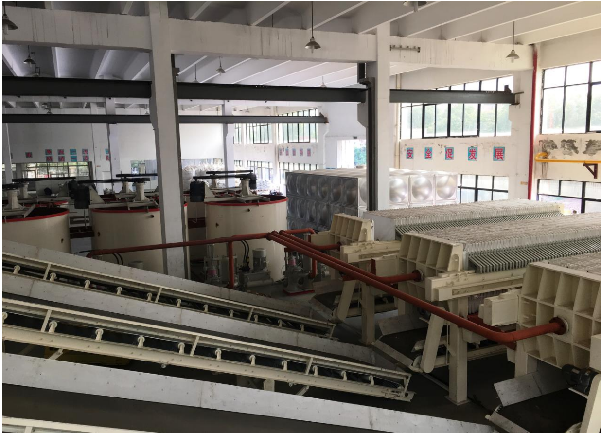
Changxing Factory – mixers, filter presses and conveyor to gas dryer
