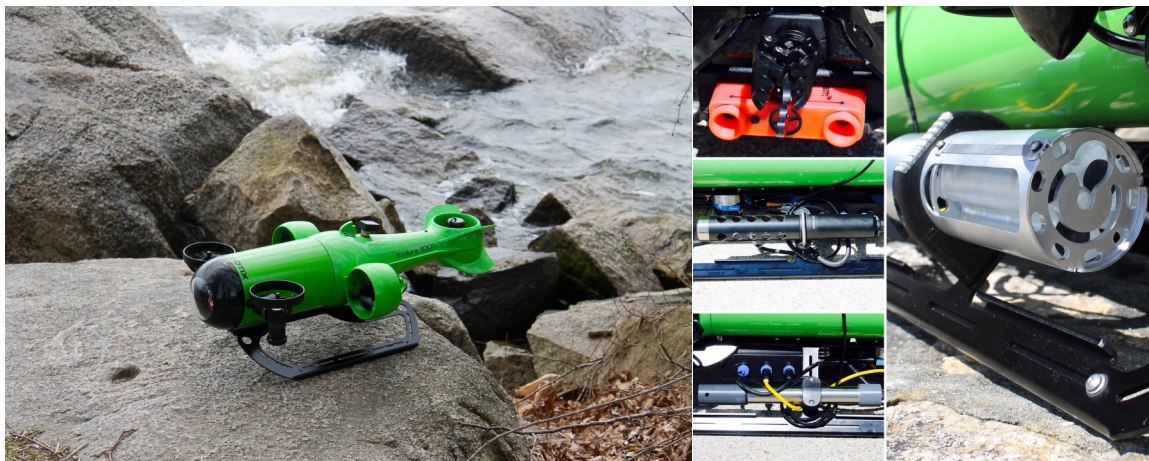
Endura 3 (left) and a range of sensors that have been integrated to the system and installed for recent deliveries, including environmental sensors, laser scaler, grabber arm and water sample collector (right)
