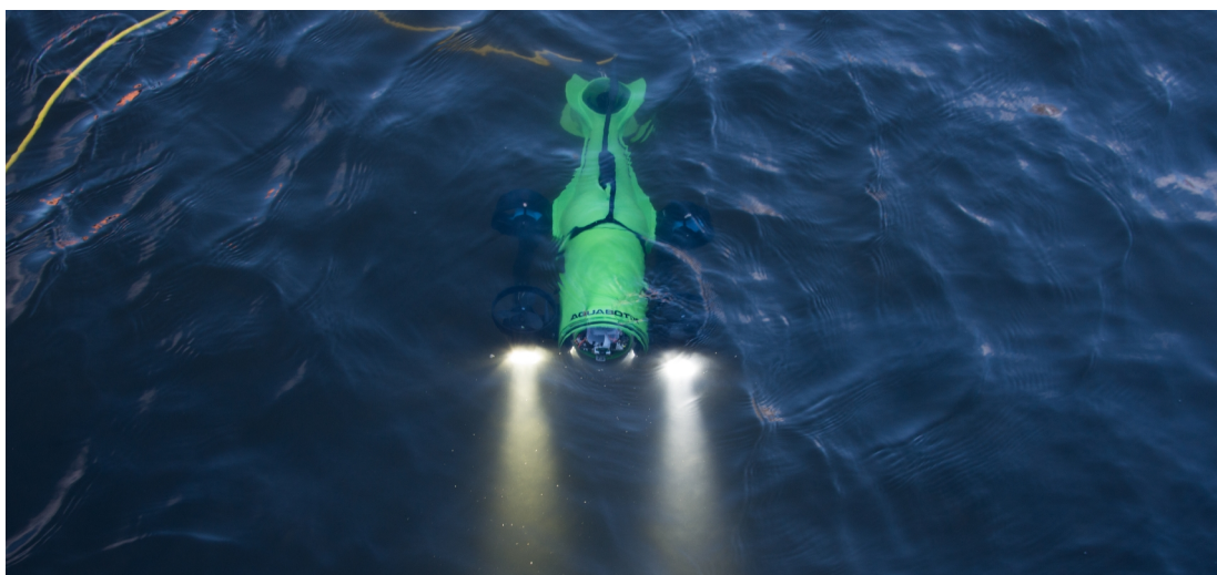
AquaBotix's Endura underwater drone approaching inspecting harbourside infrastructure
