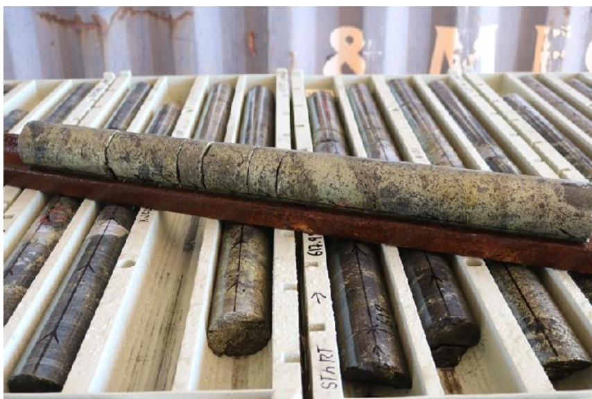
Photograph 2. Hole KJCD215 - Zone of semi-massive and breccia of magnetite + chalcopyrite (Conductor 5) circa 615.96 – 617.41 m.
