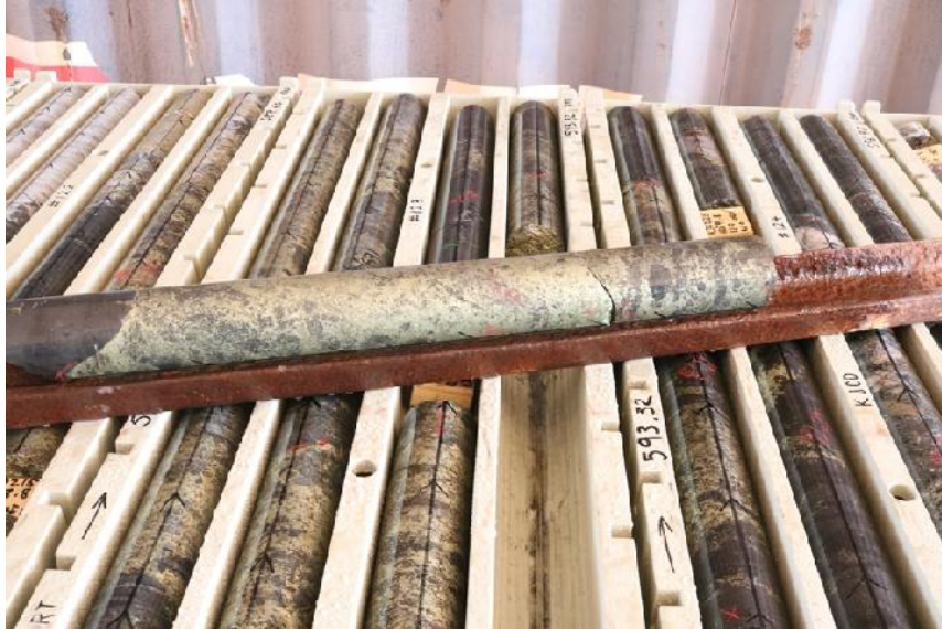
Photograph 1. Hole KJCD215 - Zone of semi-massive and breccia of magnetite + chalcopyrite (Conductor 3) circa 592.36 – 593.05 m.
