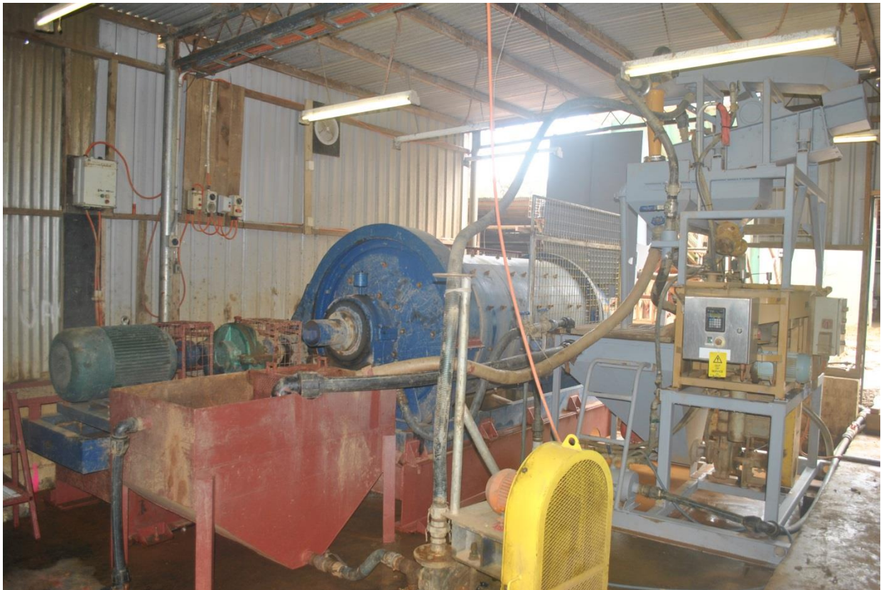
Newly installed 5 tph ball mill and concentrator
