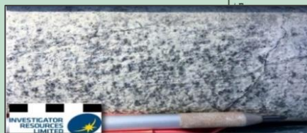
Kaolinite pyrite alteration with trace alunite topaz fluorite similar to Nankivel Hill
