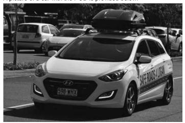
SenTAS -SenSen's state-of-theart automated traffic monitoring system. SenTAS is SenSen's automated traffic monitoring system. In essence, this system uses high-resolution cameras, thermal vision and video analytics, to accurately recognises trucks, cars, motorbikes, cyclists and pedestrians.
