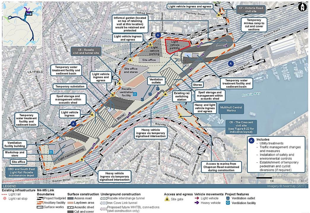
Figure 6-21 Indicative Rozelle civil and tunnel site (C5) and Victoria Road civil site (C7) layout
