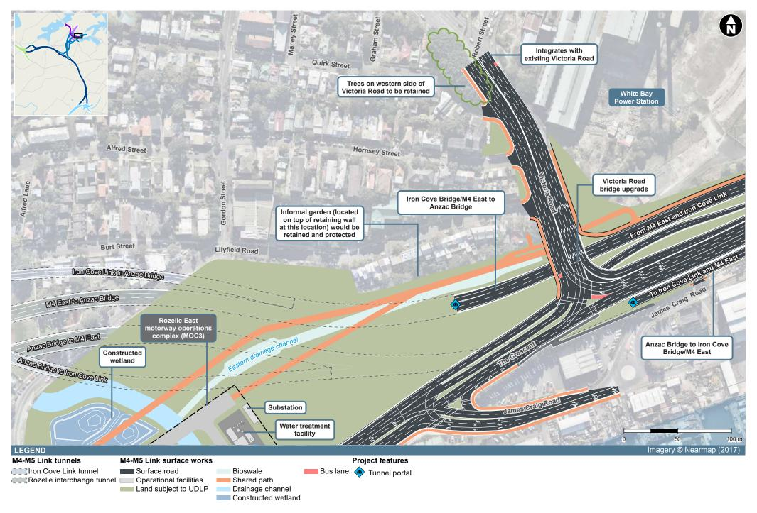
Figure 5-27 Rozelle interchange surface works overview - Map 3
