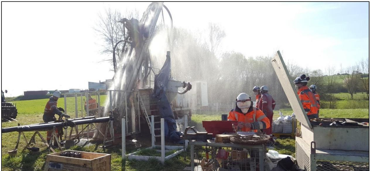
Figure 24: Reverse circulation drilling at the Belleville gold prospect south of La Bellière gold mine.
