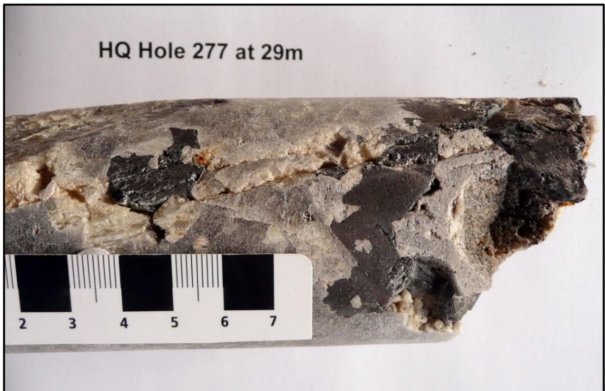
Photo 2: Hole T277C – 29m: Siliceous host rock with coarse grained tungsten (ferberite) and quartz vein. Metre interval assayed 1.23% (12,335ppm) \text{WO}_3 .
