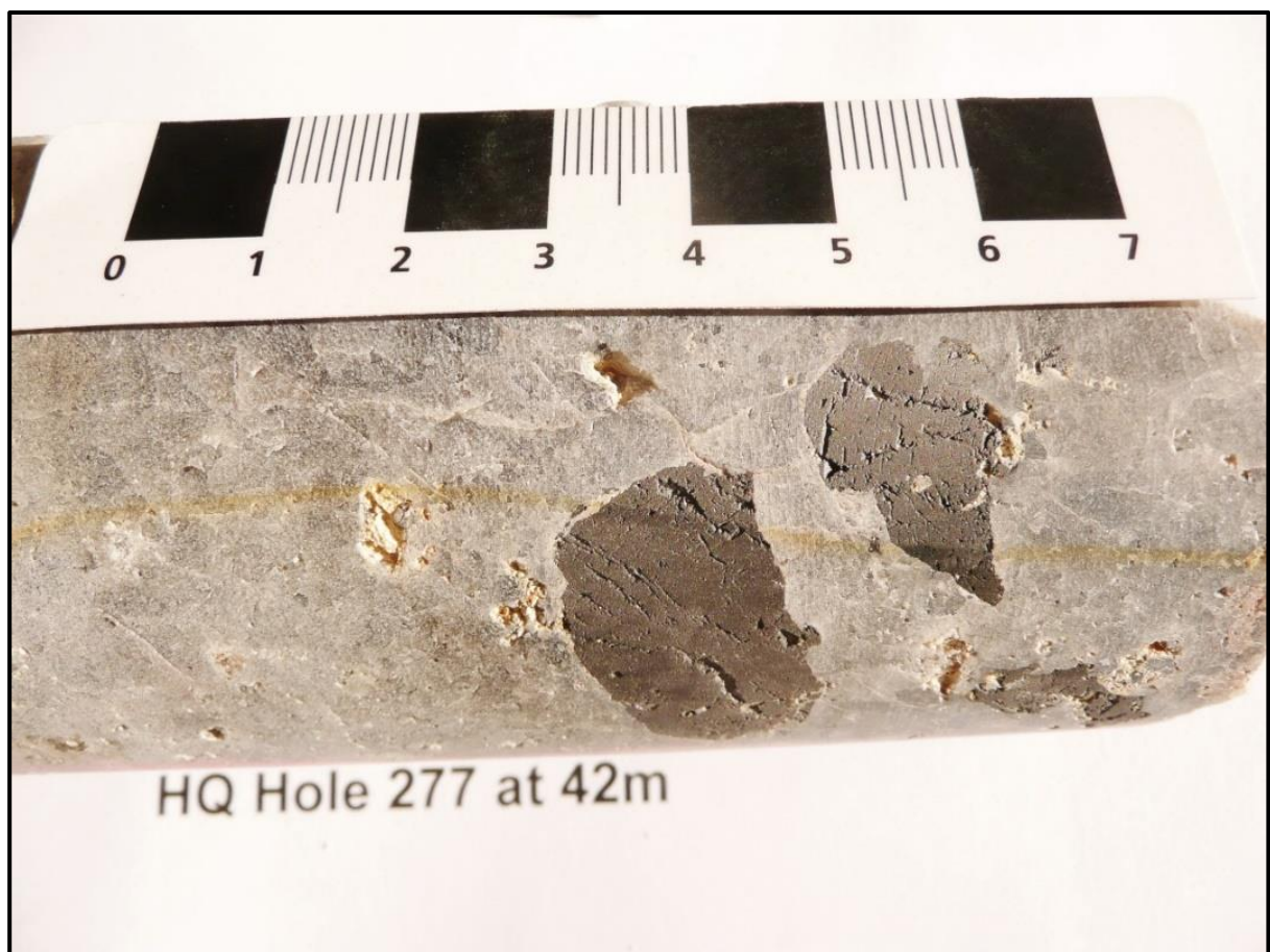
Photo 3: Hole T277C – 42m: Siliceous host rock with coarse grained tungsten mineralisation (ferberite) and white feldspar pegmatite (right). Metre interval assayed 5,405ppm \text{WO}_3 .
