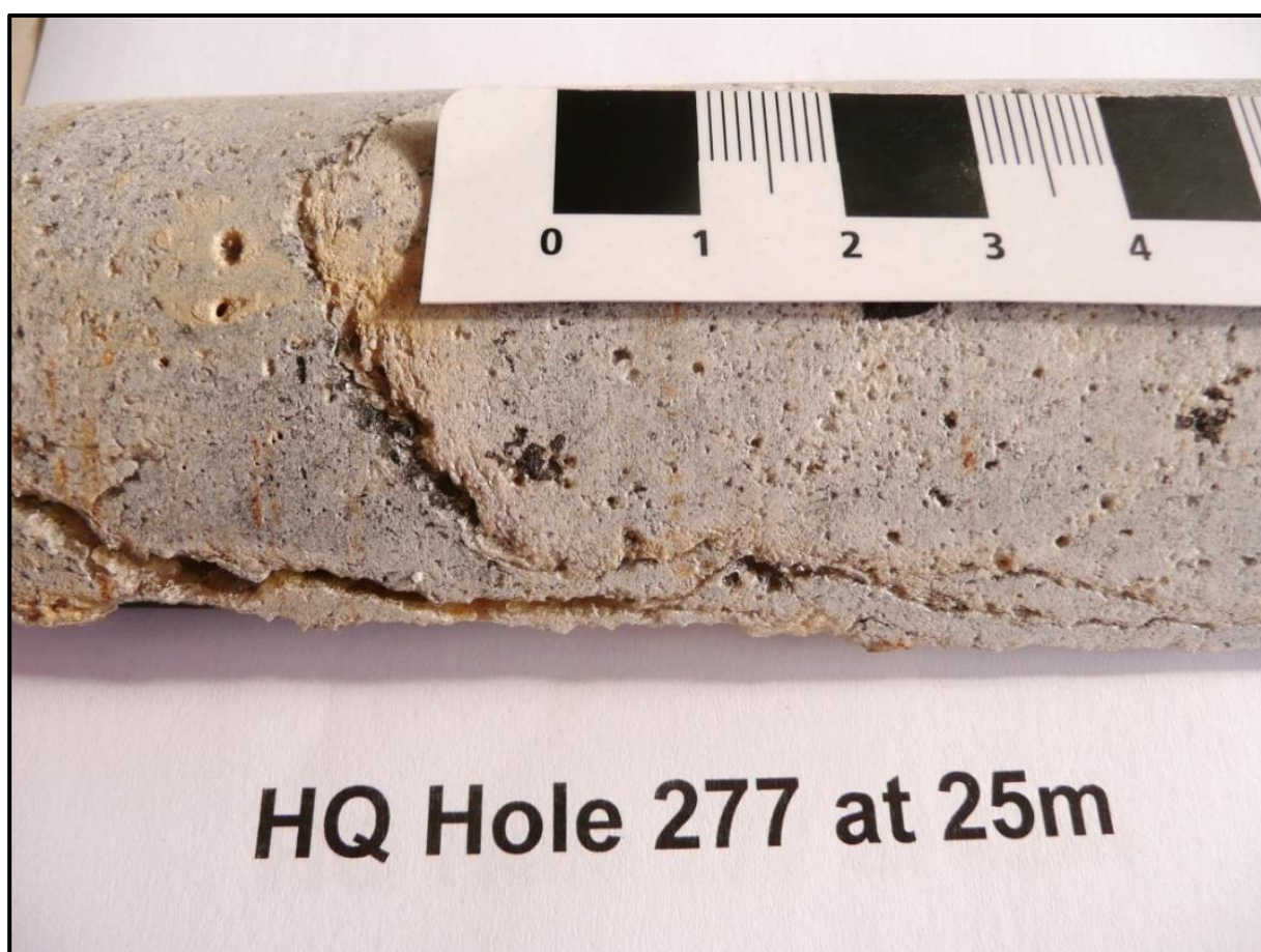
Photo 1: Hole T277C – 25m: Weathered fractured silicite with disseminated tungsten (ferberite) through silicite and on fractures. Pitting - weathered out ferberite and kaolin (muscovite). Metre interval assayed 8,618ppm WO 3 .
