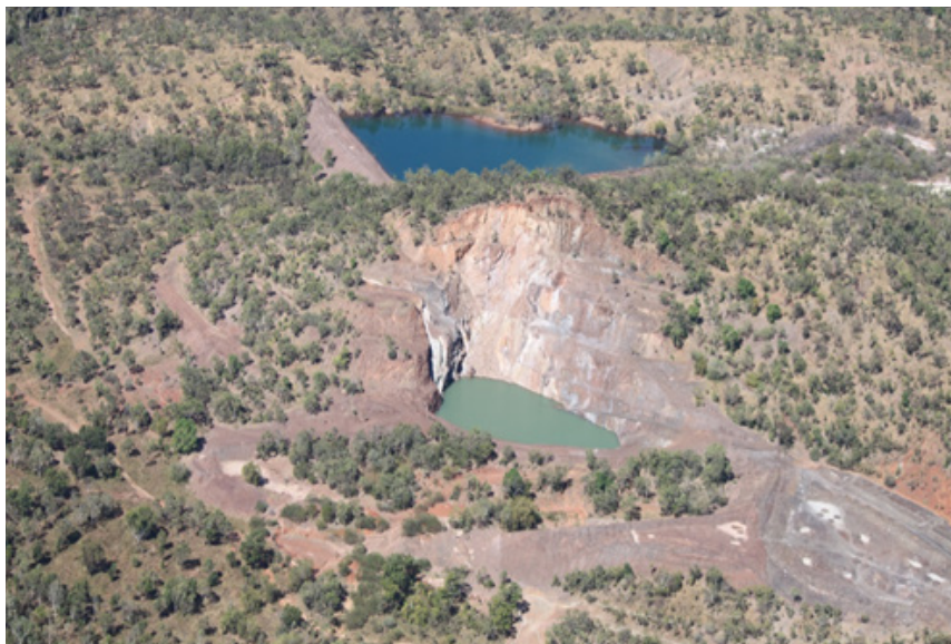
Mt Bonnie deposit aerial view (2011) looking east showing low grade stockpile in the foreground, historic open-pit centre, and water storage dam at the back
