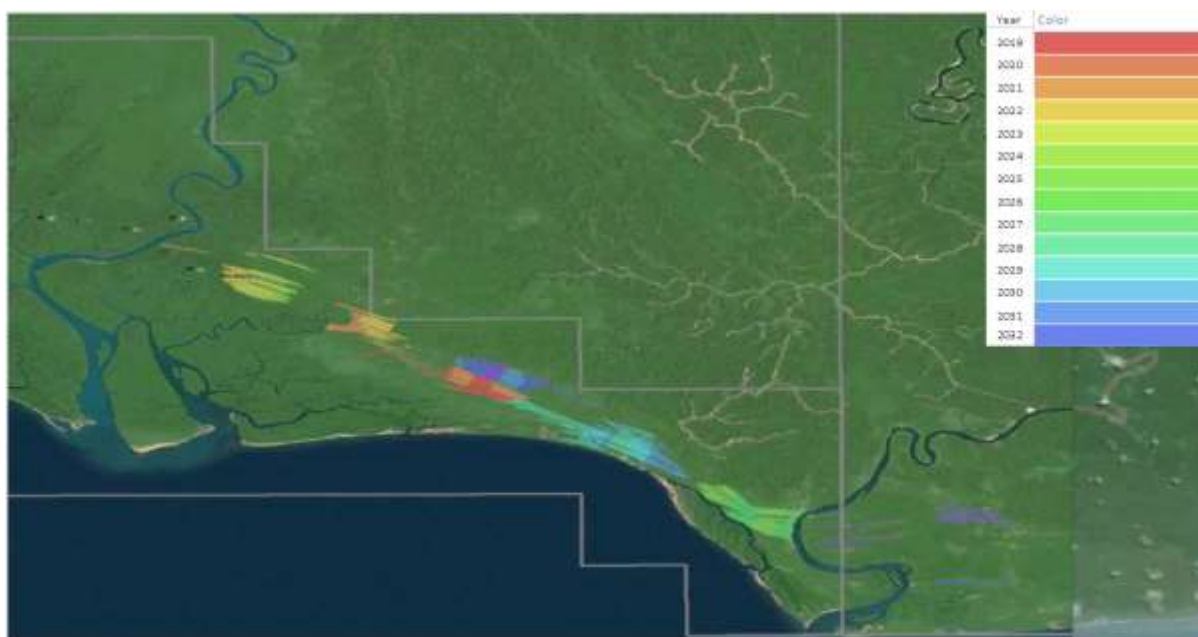
Figure 5 - Potential JORC mining Schedule by year - Excavator
