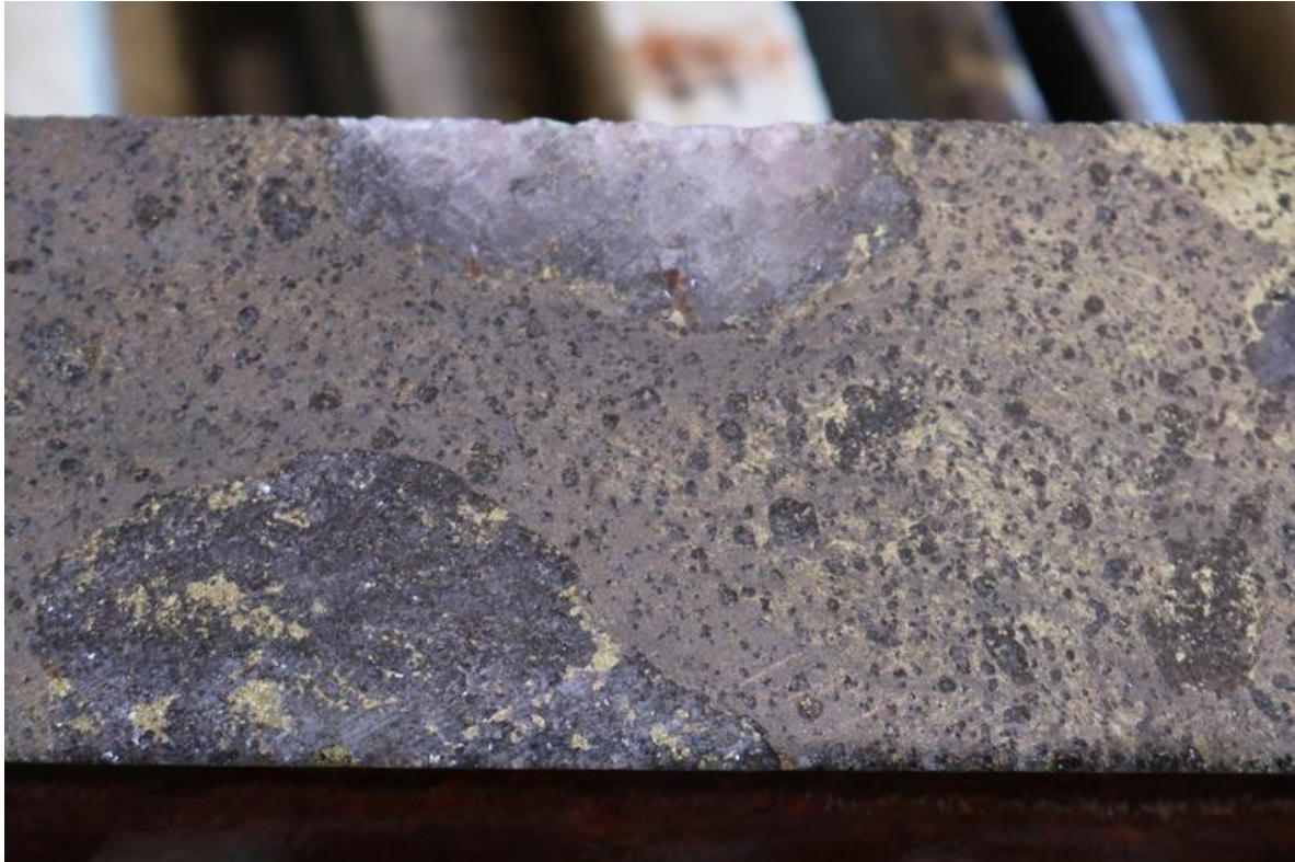
Photograph 1. Close-up of massive sulphide zone showing a breccia matrix of chalcopyrite and pyrite with fragments of rounded magnetite and quartz. Quartz shows inclusions of chalcopyrite and minor molybdenite. (KJD216 circa 645.27-646.6m)
