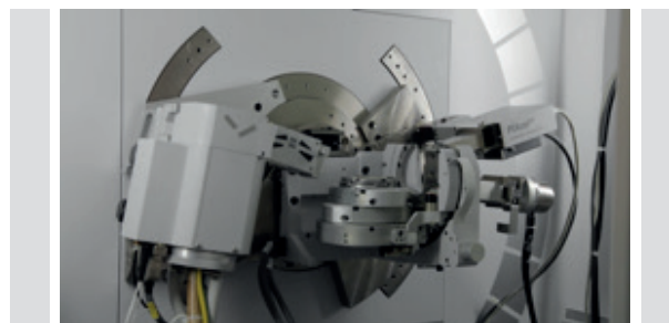
View of the X-Ray Diffraction characterisation system, which is part of the state-of-the-art characterisation and testing capabilities at BluGlass.
