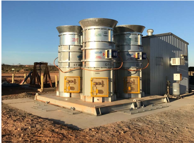
Primary fan bank at the ventilation shaft collar fully installed and running
