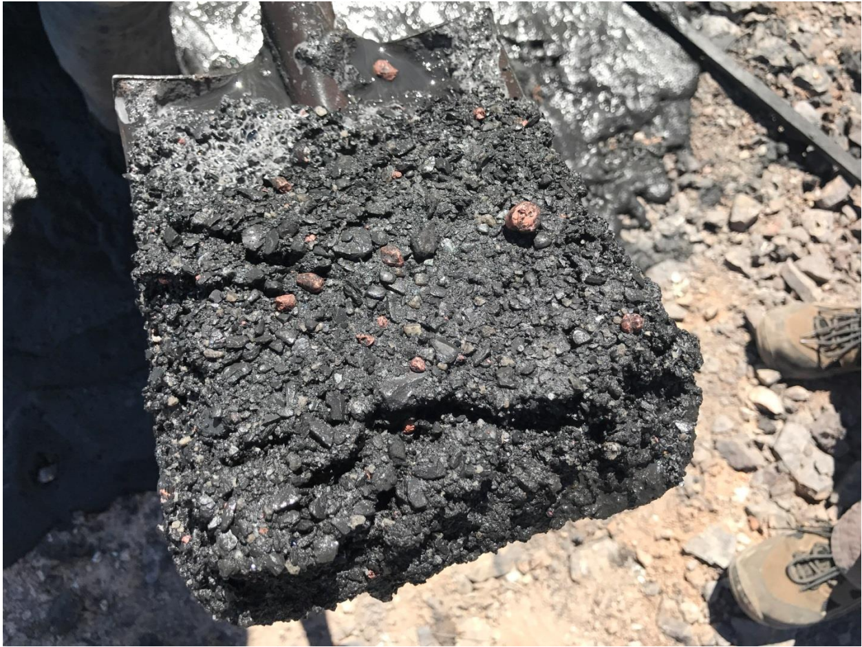
Figure 4 Native copper grains (red) exposed from drill cuttings (mostly black shale) piled under the cyclone of the RC rig
