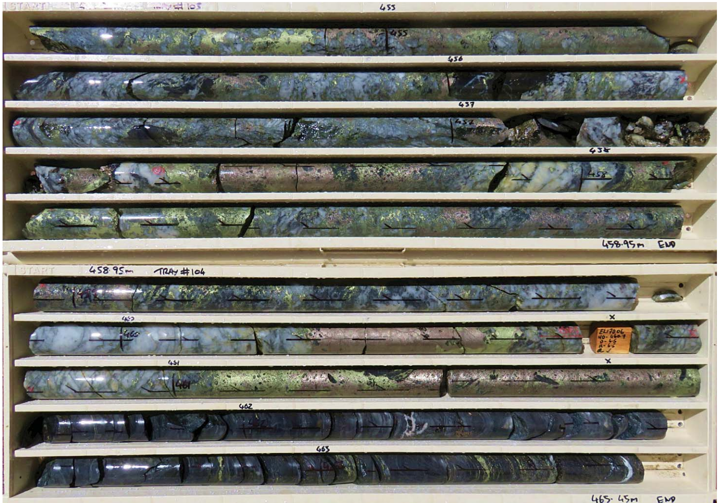
Figure 6: EL17D06: zone of massive and semi-massive sulphide between 454.5-461.7m. Sulphide is mostly chalcopyrite (yellow) with lesser pyrrhotite (bronze in colour).
