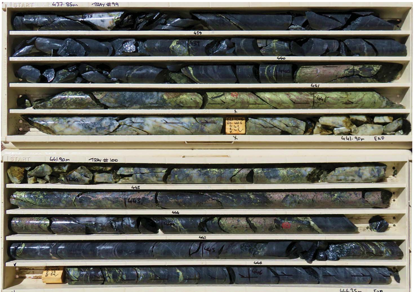
Figure 5: EL17D06: zone of massive and vein sulphide between 439-446m. Sulphide is mostly chalcopyrite (yellow) with lesser pyrrhotite (bronze in colour).
