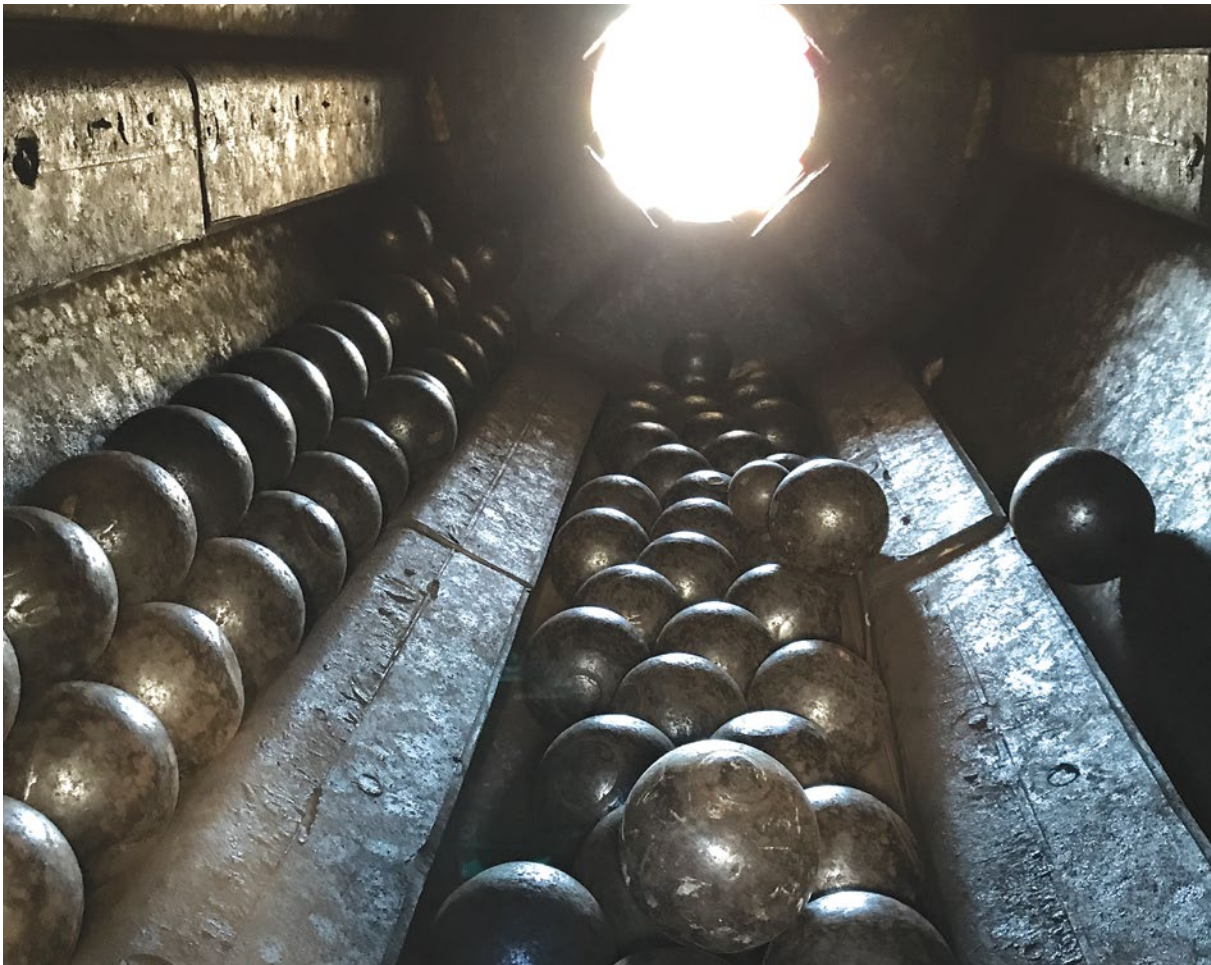
Interior of ball mill used for pulverising BOF and EAF dust to generate a slurry
