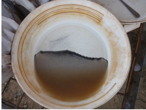
HM mineralisation present in sample from hole CB016, 21-24m depth
