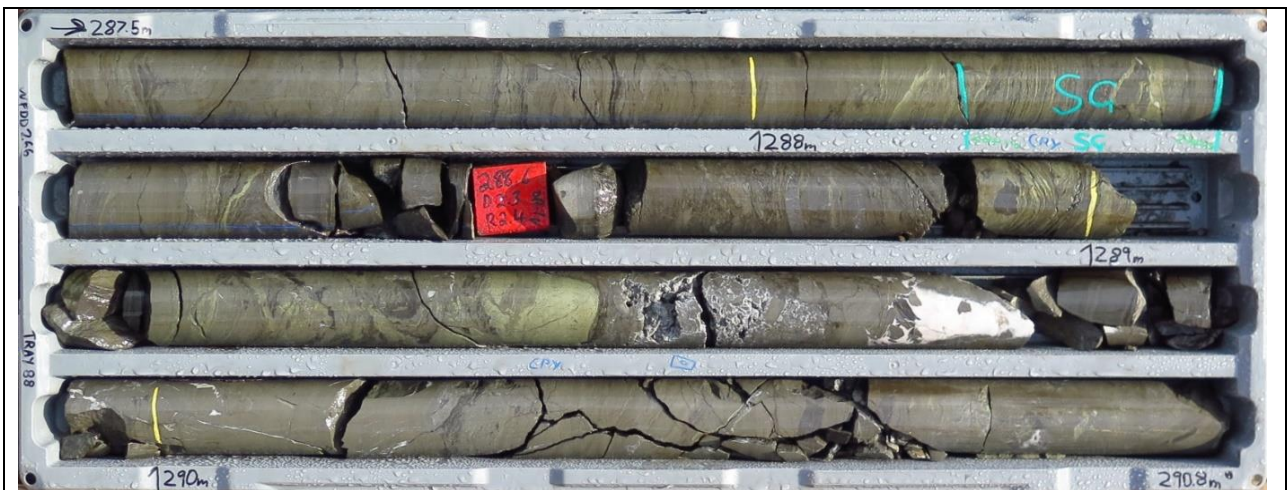
Figure 5: Tray 88 from hole WFDD266 showing strong chalcopyrite mineralisation in the Py3.
