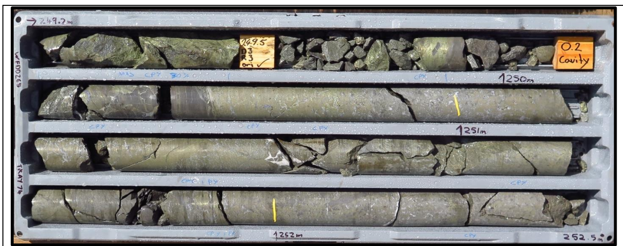
Figure 4: Tray 74 from hole WFDD265 showing strong chalcopyrite mineralisation evident overprinting pyrite zones in micrite dolomite unit at roughly 250m in Py3.
