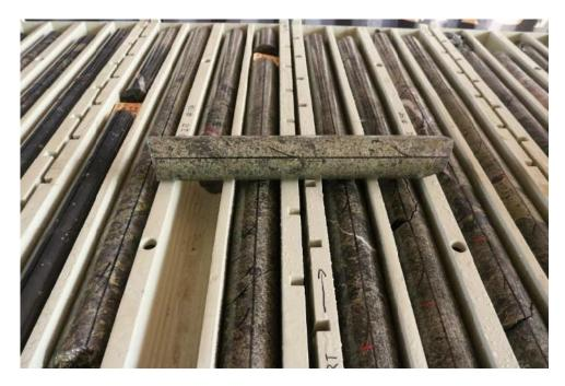
**Photograph 1.** KJCD212 - Massive sulphide zone comprised of pyrite + chalcopyrite, at 682-688.6m.
