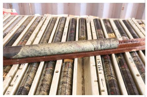
Hole KJCD215 - Zone of semi-massive and breccia of magnetite + chalcopyrite (Conductor 3) circa 592.36 - 593.05 m.
