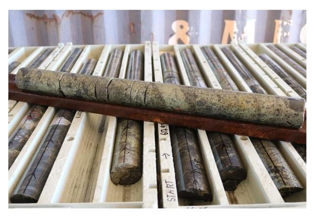
**Photograph 2.** Hole KJCD215 - Zone of semi-massive and breccia of magnetite + chalcopyrite (Conductor 5) circa 615.96 - 617.41 m.
