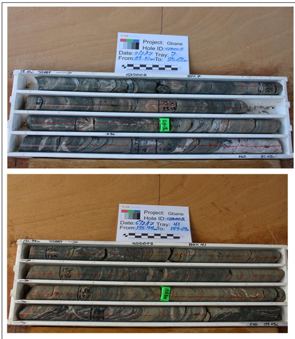
Figure 2: Core from GDD 002, showing intense shearing, alteration and quartz – carbonate veining. Intersection 24.9m to 26.3m @ 2.28g/t and intersection 136m to 139m @ 2.33g/t. Intersections are typical of the main mineralised shear zone.
