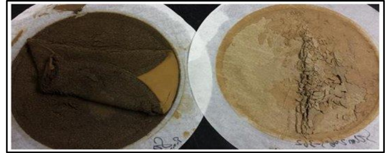
Pilot plant testing at Eriez using a rougher-cleaner flotation circuit. Difference in colour of the tails on the left and the concentrate on the right demonstrate the effect of the cleaner stage
