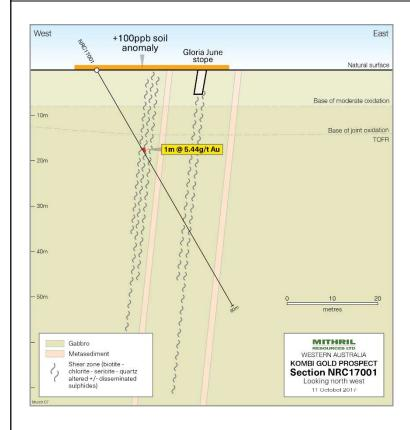
Kombi Gold Prospect – NRC17001 (left) and NRC17004 (right) cross sections. Sections shown at same scale approximately 100 metres apart
