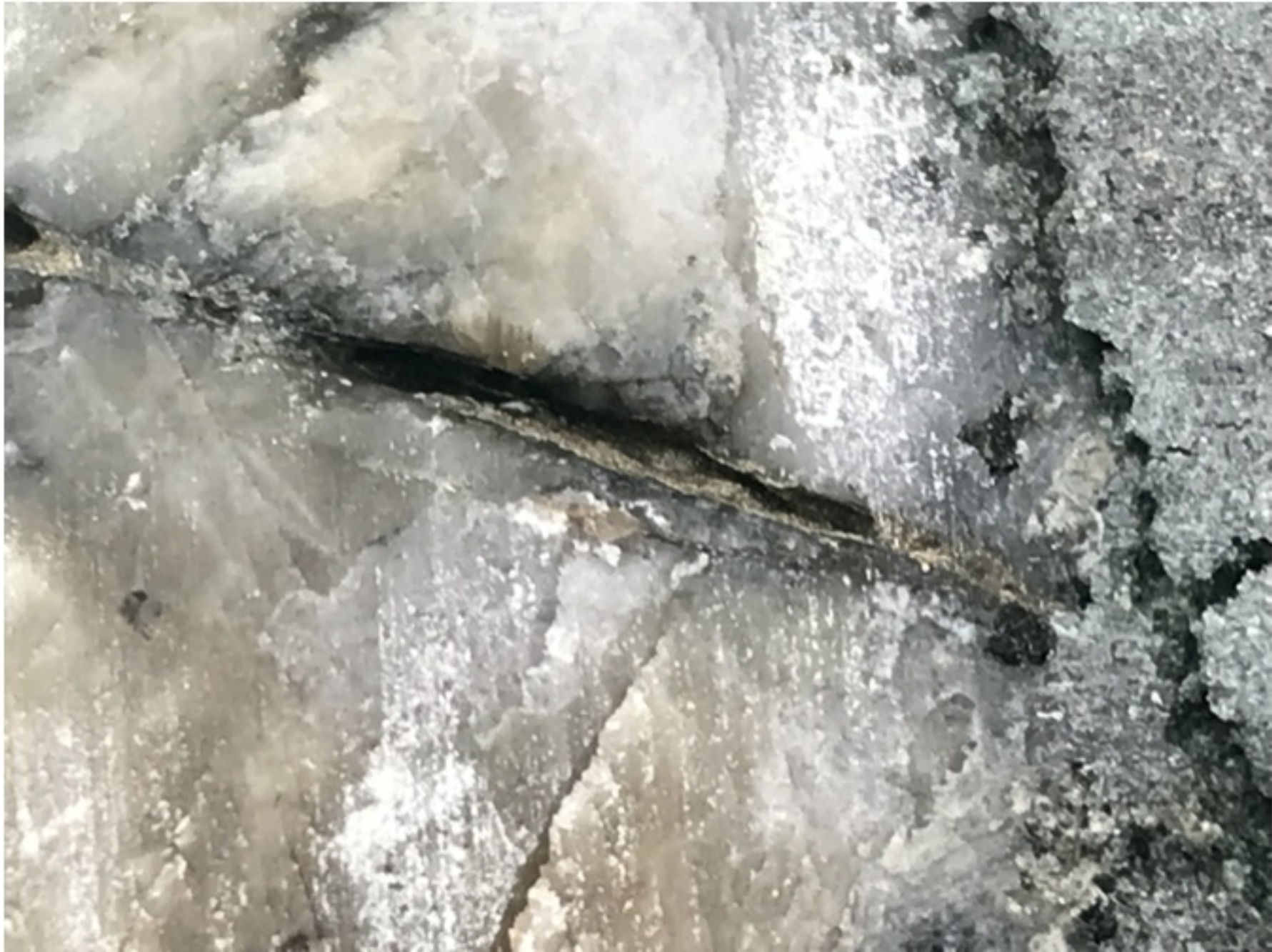
Figure 4: Pyrite-rich fracture in quartz-tourmaline vein – Hole 17ATDD002 (from 39.5m)
